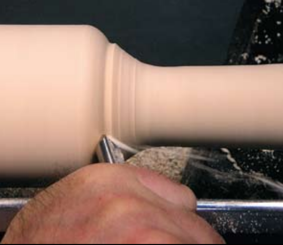
Figure 7 – Make a sliding entry from the top with a gouge . You can form the entire bead with the gouge, but the inside corner will not be sharp.
