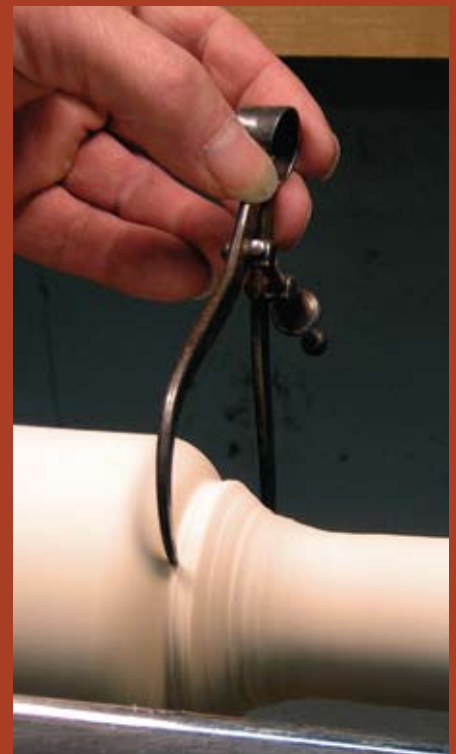
Figure 6 – After roughing with a gouge, check the diameter of the shoulder with a caliper
