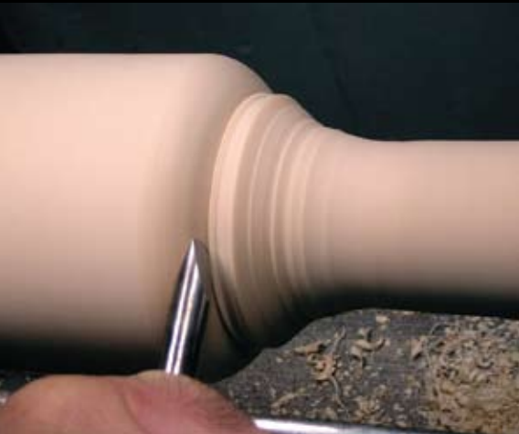
Figure 8 – Slice through the grain holding the skew chisel almost vertically. Round chisels, as shown here, work well for small details.
