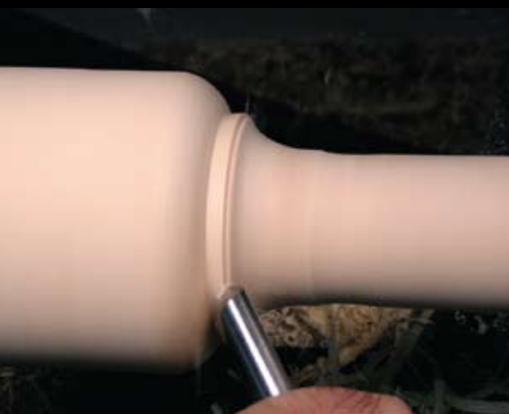
Figure 10 – The accurate placement of the gouge establishes the width of the shoulder.
