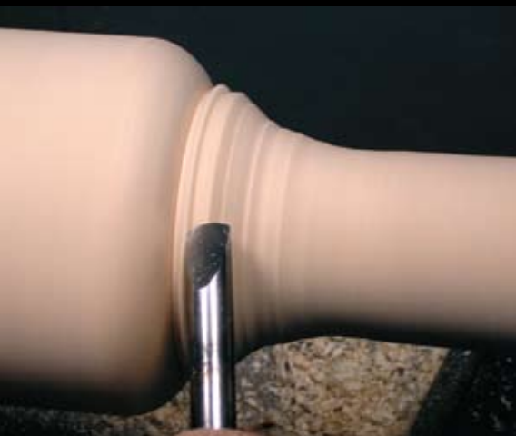
Figure 9 – Enter with a skew chisel from the side and make a planing cut.
