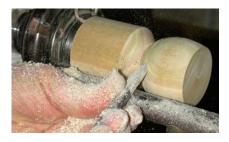
Now, shape the outside of the egg-cup bowl. Use the spindle gouge to create your own details at the rim of the bowl and at the base of the bowl. Leave enough stock at the bottom of the bowl to support hollowing the interior. *Above* are 10 profiles for idea starters.
