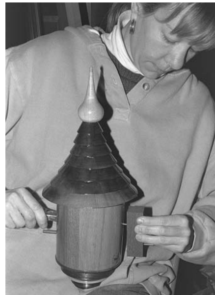
Screw the birdhouse to the mounting bracket through the house's opening.
