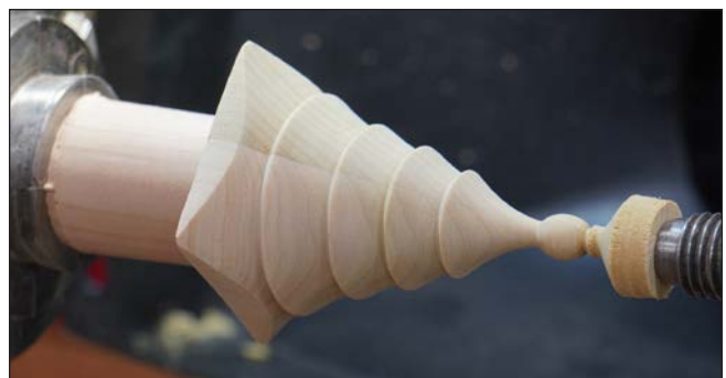
Photo 12. After remounting the roof blank, turn the roof details, taking care not to cut into the 3/4" hole drilled in the previous step.
