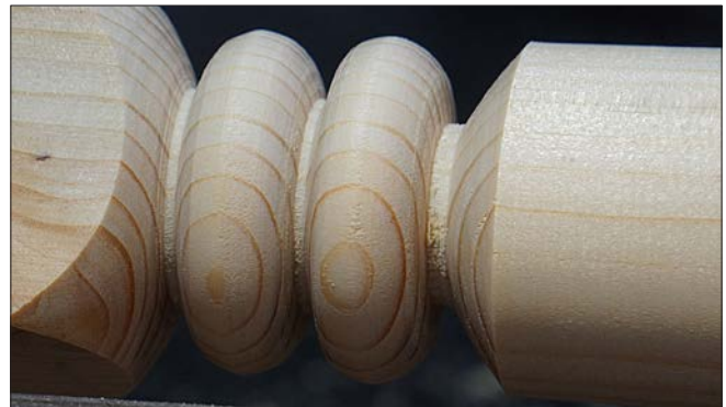
Photos 3-4. Subtle details grace these forms, including a lamb's tongue transition from round-to-square features (left). If the beads will be painted, a small cove (or flat) between them will make decoration easier.
