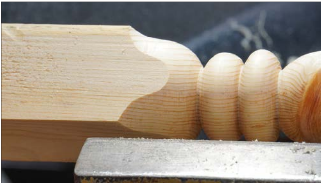
Photos 3-4. Subtle details grace these forms, including a lamb's tongue transition from round-to-square features (left). If the beads will be painted, a small cove (or flat) between them will make decoration easier.
