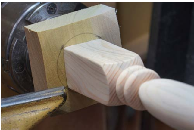
Photo 8. To maintain a flat mounting surface for the spindle, mark the perimeter of the spindle on the base.
