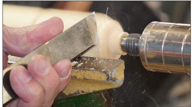
Photo 2. Round over the top of the bird house to meet the tenon using the heel of the skew.
