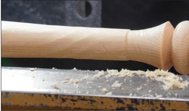
Photo 5. Chatter appears as the stock becomes thinner and the cut is farthest from tail- and headstock support.
