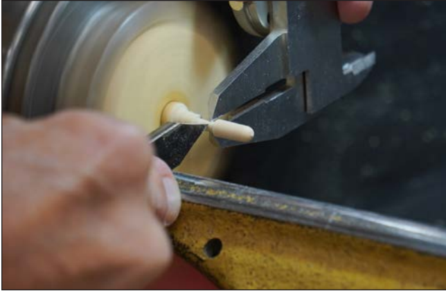
Photo 6. Turn the perch either from a dowel or a prepared blank with a 3/8" tenon glued into a waste block.
