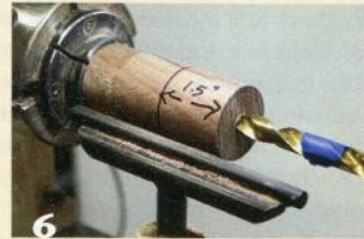
Drill a hole to aid in hollowing. Masking tape on the drill bit provides a visual guide to confirm drilling depth.
