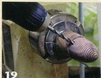
19 Drill an "entrance hole" near the base of the beehive.
