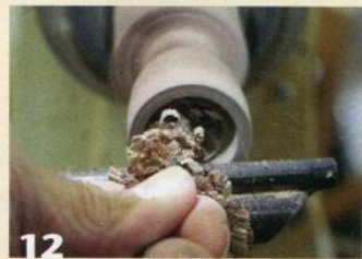
The author hollows the endgrain form using a spindle gouge, pulling the tool from center hole left to the outer wall.
