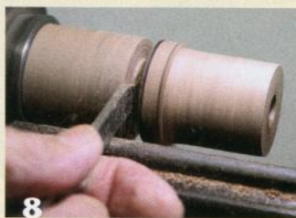
An additional line indicates overall height of the beehive. Make a parting cut here but leave enough material for support during hollowing.
