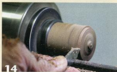
14 Make a jam chuck of the wasteblock remaining in the chuck. Glue the beehive onto the tenon of the jam chuck. A portion of the wasteblock will become the bottom of the beehive.
