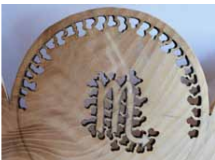
Photo 29 Try to Maintain An Even Wall Thickness
