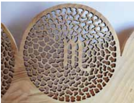
Photo 32 Sand with 400 Grit to Remove Marks
