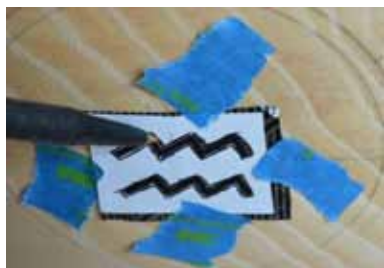
Photo 16 Applying Image with Carbon Paper
