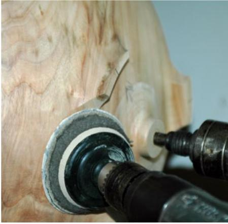
**Photo 15** Finish sanding to 320 with soft pad
