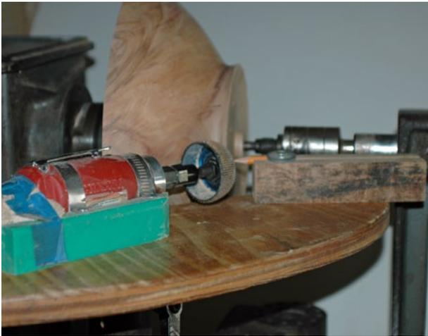
**Photo 7** Use of a table and air grinder sled for carving
