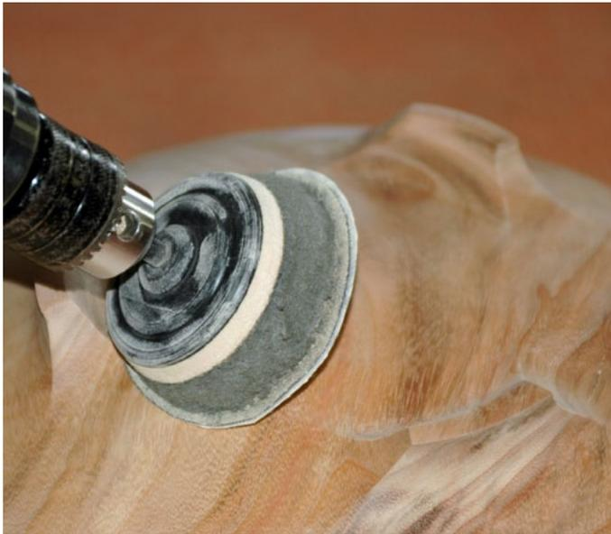
**Photo 19** Finish sanding to 320 with soft pad
