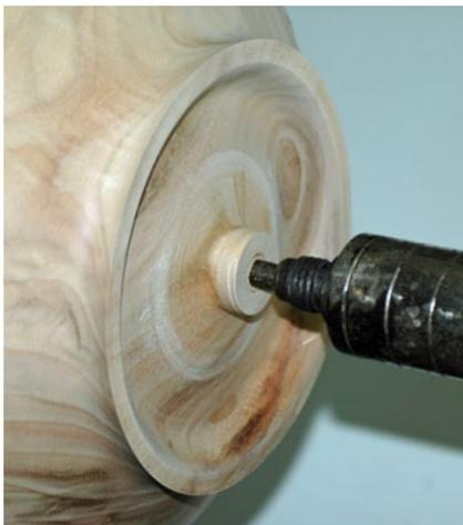
**Photo 6** Turning the inside of the foot ring
