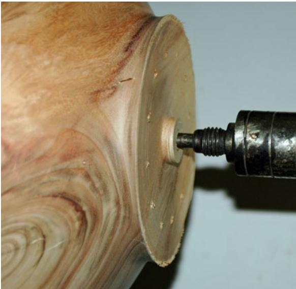
**Photo 5** Use of centering pin for reverse turning
