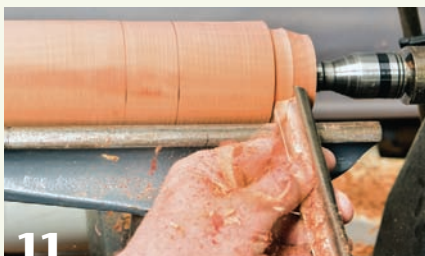
11 Mark all transitions and rough to just over finished diameter. A partially turned bottom tenon acts as a sizing gauge when turning the bead.
