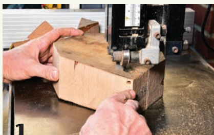
1 Cut the top and base blanks to size on a bandsaw and remove the corners to speed turning. Take extra care if the blank is cupped or warped.
