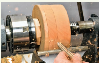
3 Using a bowl gouge, turn the top round, cutting in from both sides to avoid tearout. Then true up both faces.
