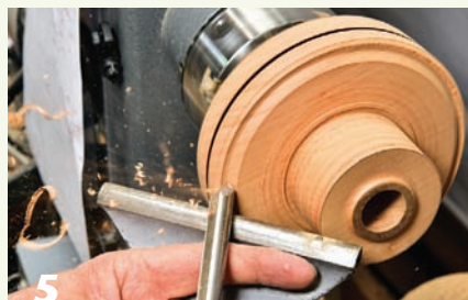
5 Using a bowl gouge, turn a spigot from which you will create a bead. Then start the ogee shape on the underside of the top.
