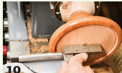
10 Part in to depth, then shape the recess with a gouge and scraper. Check for flatness with a small square.
