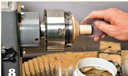
8 Make a chucking spigot to reverse-mount and turn the top and base. Fine-tune the spigot with abrasives for a snug fit.
