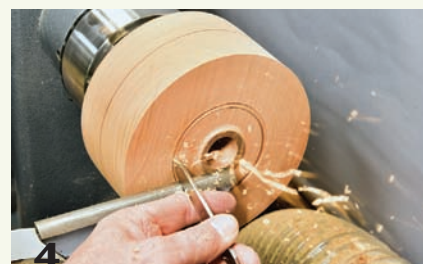
4 Drill a hole, or mortise, that will later accept the tenon at the top end of the stem. Mark, then plunge in with a small parting tool to indicate both the position and, where possible, the depth of key transitions.
