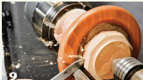
9 Reverse-mount the top on the spigot drive, and bring up the tailstock for support. Part off the original glueblock.
