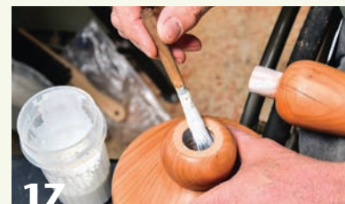
Apply glue to the mortise and tenon only to prevent excessive glue squeeze-out.
