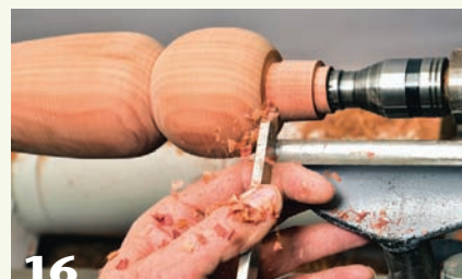
16 Turn the tenons to their final diameter for a snug fit in the drilled mortises.
