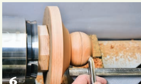
6 Mark the center of the bead, then shape the bead with a spindle gouge. Then further refine the ogee to the left.
