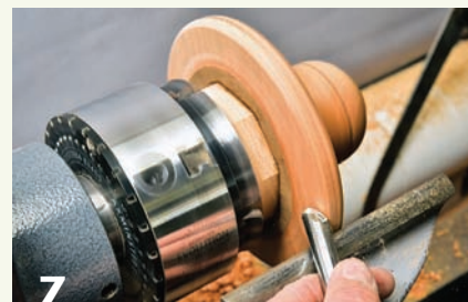
7 Using the lower wing of a bowl gouge presented on its side, create the bead, or roundover, at the top's largest diameter.
