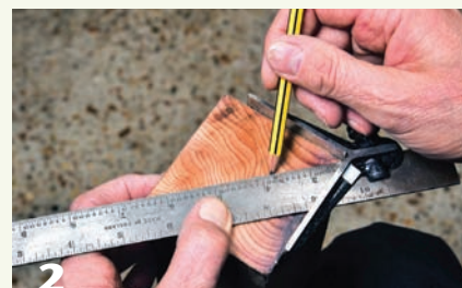
2 On spindle blanks, mark the center line from all four corners, then eyeball the middle and center punch.
