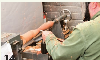
14 Mark your toolrest to indicate the center of the narrowest point on the stem, as a mark on the wood would be turned away. Rough down from both sides.
