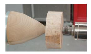
Mount your blank between centers onto the tenon and support with the tailstock. If the piece is loose apply a small piece of masking tape onto the tenon in order to tighten it.
