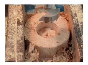
Tea lights come in a number of different diameters so buy your candles before you start the drilling part of this project. In my case I'll drill a hole 5/8" deep and 1-9/16" diameter in the center of your blank. A drill press with a vise attached is very handy as it is quite important to drill a nice clean hole.
