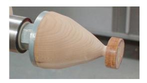
In order to mount this blank on my lathe I've turned a waste block with a 1-9/16" tenon at the end which will be used like a jam chuck to hold the blank in place. Note that I've tapered my waste block down considerably to provide me with the space to turn and sand the top of the tea light.
