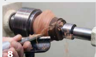
8 Reverse the blank in the chuck, holding it once more in expansion mode, and shape the lower section of the candleholder. The author uses a gouge, followed by a negative-rake scraper to refine the surface.
