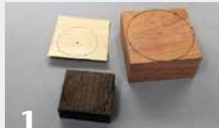
1 The blank comprises three contrasting pieces laminated together. Use a compass to draw a circle on each for trimming on the bandsaw.
