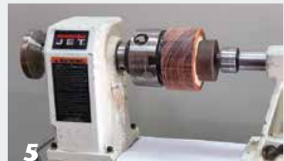
5 The lathe is an excellent clamping device. Use the tailstock to apply pressure during glue-up. Note the veneer is sandwiched between the top and base sections.
