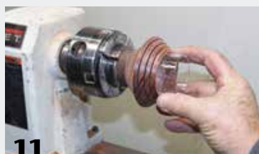
11 Test fit the glass cup and fine-tune the fit if necessary. Sand the work.
