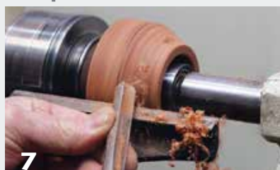
7 With the piece reversed and now held by the base tenon, shape the top section. The author forms an angle from center to the top rim.
