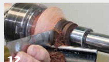
12 Reverse the piece in the chuck one last time, and part the tenon from the base. Complete and sand the bottom.
