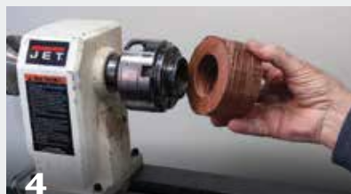
4 Use the drilled hole to mount the top section on a chuck in expansion mode.
