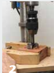
2 In the thickest piece, drill a hole for the glass cup. Trim the pieces round. The veneer can be trimmed using scissors.
