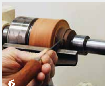
6 After the glue dries, form a tenon at the base to fit in your chuck jaws.
