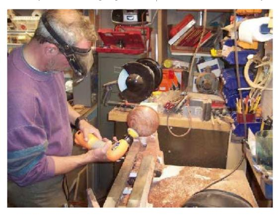
Just a sanding pic. Using my cheap Harbor Freight angle sander, It works good though. I sand up to 320 or 400 grit.
