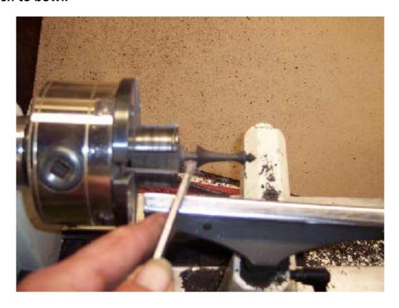
The reason I'm using these jaws is cause on this bowl instead of having a straight foot I made the outside into a half bead. If I made a full bead I wouldn't have been able to hold it in my chuck. So the foot curves to the outside & the inside is straight sided. Also my other jaws wouldn't close far enough so I had to change jaws.
