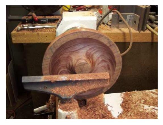
I want it to flow nicely from the top to a gradually flow into the base of the bowl. I want the slope of the center to approximately mirror the slope of the outer edge of the bowl. I also finish the rim type I want. This one has some fabulous grain pattern I'm very pleased.
