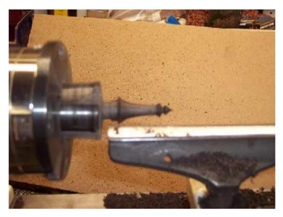
Just double checking the final size of both the base of the finial & of the tenon to make sure I didn't screw up.
