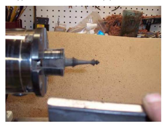
Here I am turning down to the final size tenon. I like to go with at least 3/16" - 1/4" tenon for strength. (I broke one before cause I made it to thin just inserting it into the bowl)
