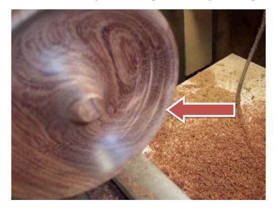
finished sanding & the bowl is a little under 6" now you can see how the center flows from the top to gradually go into the bottom. & there is plenty of room for bracelets etc...
