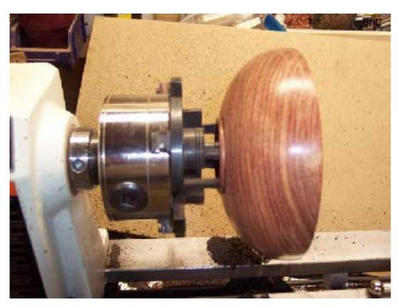
Here I put tape so I know when I reach my final depth. I like to make the length of the tenon about 1/4" - 3/8" so I have a decent amount of gluing area.
