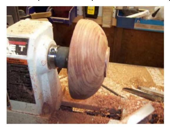
I take a 2" hook & loop sanding disc to sand around the foot so I can get right to the edge.
