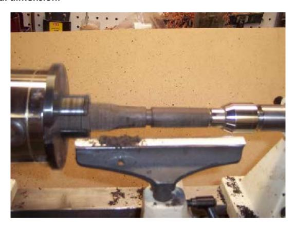
Well the finial is finished. I also snuck up on the dimension of the center part. I just took about 3/16" more under the base but left enough for sanding. The tenon part is about 3/8" right now.
