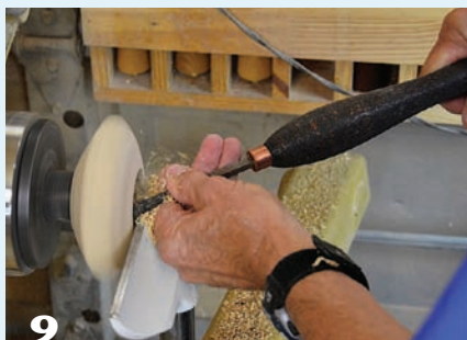
9 To hollow smoothly with a bent-tip tool, position the toolrest slightly above the lathe axis and raise the tool handle.
