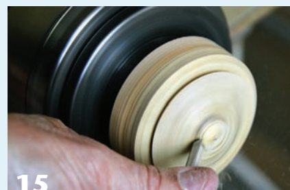
15 Remount the lid in a jam chuck so you can cut a gentle ogee on its top surface.
