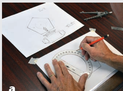
a Using compass, straightedge, and protractor, you can draw regular polygons of any size with any number of sides.
