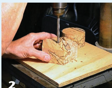
2 Center-bore the blank for mounting on a worm screw held in a scroll chuck.
