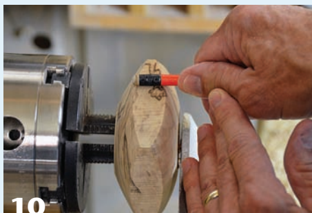
10 Gauge the depth of the vessel with a pencil and aim for a \frac{3}{16} " (5mm) bottom thickness.
