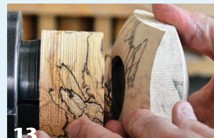
13 Check the fit often by offering the box opening up to the lid tenon.
