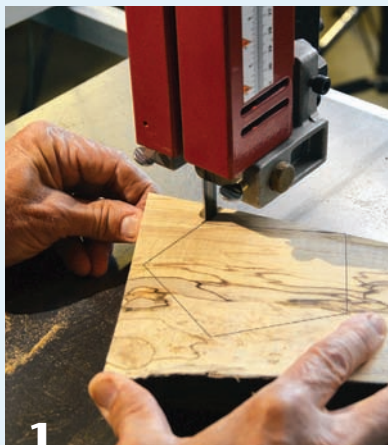
1 Carefully saw the polygonal blank. Saw just outside the layout lines.
