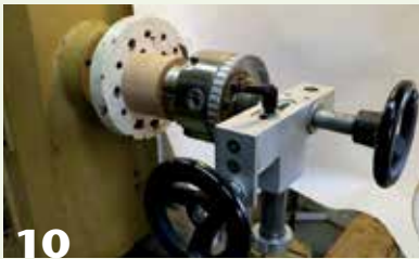
10 The author uses a faceplate to square the jig to the lathe spindle before cutting the inside threads on the mortise ring. When the blank is flush against the faceplate and the banjo is square to the lathe bed, the jig is then locked into alignment.
