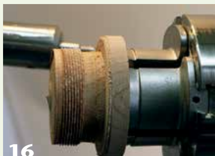
After cutting the exterior threads on the tenon ring, the author tests the fit of the mortise ring. A light sanding of the threads can loosen a tight fit.
