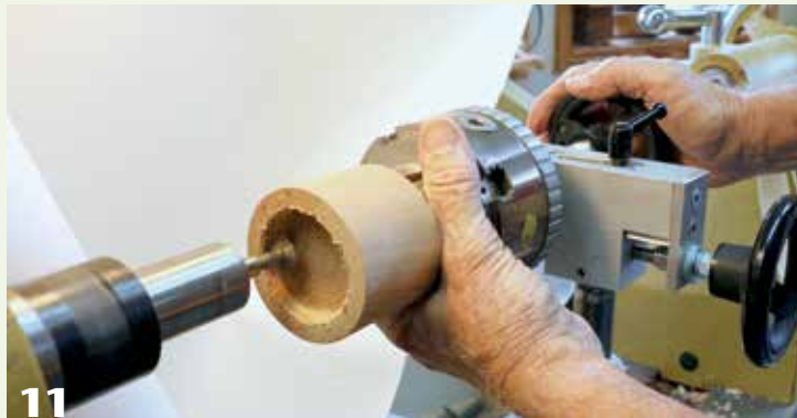
Cut the interior threads in the mortise ring.
