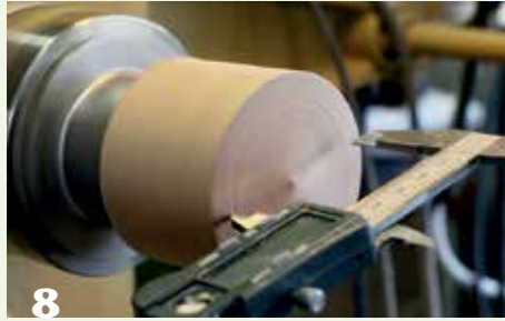
8 Use one leg of the caliper to mark what will become the inside diameter of the mortise ring, about 1/8" smaller than the desired OD of the tenon ring. Form a straight-walled recess at this mark.
