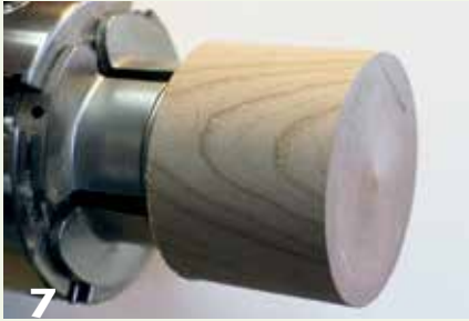
7 Turn the insert blank to the inside diameter of the lid.
