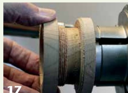
After cutting the exterior threads on the tenon ring, the author tests the fit of the mortise ring. A light sanding of the threads can loosen a tight fit.
