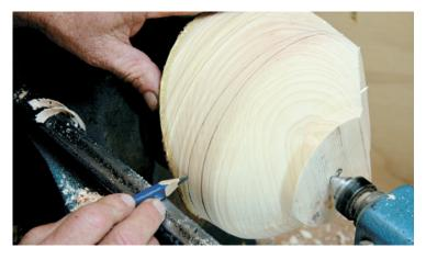
I use the same gouge to cut in from the rim, then find it easiest to fare the two cuts shear scraping with a skewed scraper (photo 10). Shear scraping generally produces the best surface working the bark sections (where there is more space than wood). By taking a series of short back and forth shear scraping cuts that remove only dust or diaphanous ribbons you can minimise tool pressure against the wood as it passes more easily than when using a gouge.
