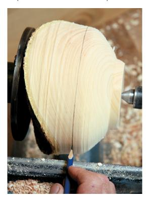
With the alignment completed finish the profile: shear cut from the base up to the bark, then in from the rim for the upper section. For these cuts I use a 3/8" deep-fluted bowl gouge with a steep right wing that enables me to start cutting just above the foot (photo 9).
