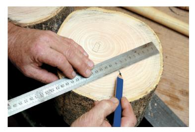
Then (photo 1) position a ruler so the bark forms a symmetrical arch over a line the length of the log (here 180mm) and mark centre. Each end of the line must reach the bark. At centre draw a line at right angles to the first line, then another parallel to the first that will define the base of the bowl. Then sketch in the sides.
