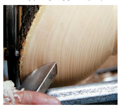
Once you have the rim an even thickness and as thin as you want it, complete the hollowing. When making the earlier roughing cuts I ensure each is slightly shorter than the last, creating a series of shoulders against which the gouge bevel can be presented for starting subsequent cuts. It makes life a lot easier.
