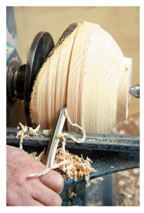
Every time you relocate the tail centre you scribe another line between the two low points to check (photo 8). Aim to have the both low points touch the line in the same manner. If you are using a small spur drive that allows the blank to pivot in more than one plane, you need to check the upper points of the rim using the same technique, except that you'll not be scribing a line as there's no wood between the two points on that plane. Note how the tail centre has been repositioned.
