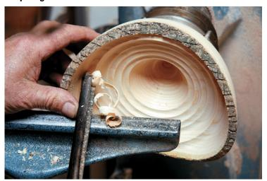
The best tool for the remounting a bowl so you can complete the base is a vacuum chuck that I don't have because mostly I've worked burl with holes in. I've always used jam chucks, and this is typical. This chuck is a roughed out bowl mounted over Vicmarc Step Jaws (photo 14).
