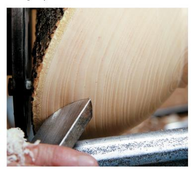
I remove most of the waste with the bowl gouge, but complete the curve into the base using a large scraper with a slight radius (photo 12).
