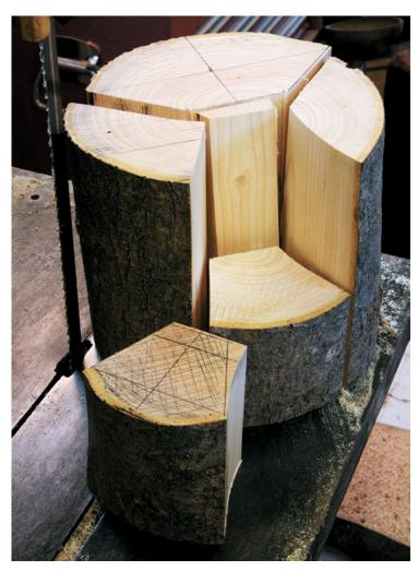
Keeping the log on end, use a bandsaw to make a series of cuts, slicing the log like a cake (photo 3). Logs too tall for your bandsaw have to be fixed bark up in some sort of sawhorse then cut using a hand or chainsaw. Or if the grain is straight you might be able to cleave the log into suitable billets: something I could have done with this claret ash.
