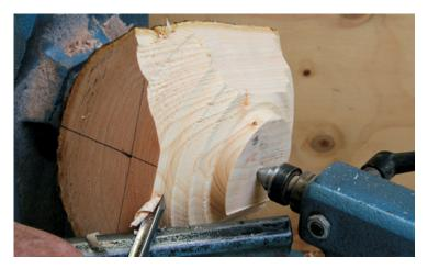
When you have the bark section trued, it's time to assess the alignment of the blank. Hold a pencil at the base of the bark on the lower of the two sides and rotate the wood by hand to scribe a line around to the other side (photo 7), which in this case is about 15mm higher. Typically you need to move the tailcentre about one third to half the gap to bring the two low points into the same plane.
