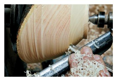
In (photo 11) you see a 1/2" nch deep-fluted bowl gouge in action. It helps to have your fingers supporting the wood to reduce vibration, and keep your hand on the rest. For the final cut for the wings I prefer the lighter 3/8" gouge I used to complete the profile.
