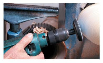
As on the profile, the wings are best power sanded to preserve the even wall thickness, (photo 13).
