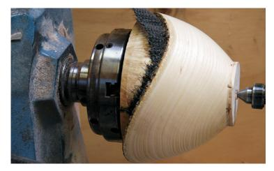
The remaining nub can be chiselled away and sanded away from the lathe, but I find that the bowl is usually on the chuck securely enough that I can finish the base using the small gouge on the lathe (photo 17)—making sure that my hand is around the bowl at all times, just in case.
