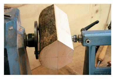
Work the bark section from the upper face as in (photo 6), so that fibres below support the fibres you're cutting. These are roughing cuts where the bevel doesn't rub the wood, hence the ridged but cleanly cut surface.
