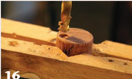
16 Drill holes near the edge of both tubes to accept recessed magnets, which provide a hidden method of holding the box closed.
