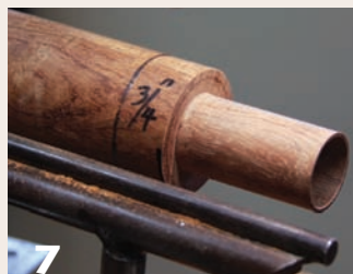
Indicate a section that will become the top of the inner tube. This is a good place for design elements such as beads, coves, or burn lines.
