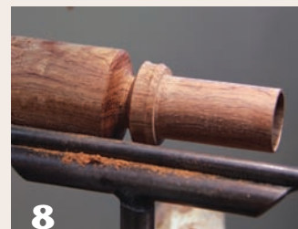
Indicate a section that will become the top of the inner tube. This is a good place for design elements such as beads, coves, or burn lines.
