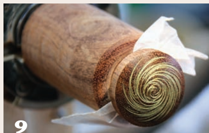
Use a hole drilled into the outer tube as a jam chuck to hold the inner tube for finish-turning its top. If the fit is too loose, add a layer of paper towel to take up the extra space.
