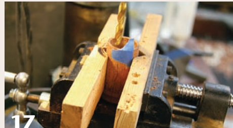
16 Drill holes near the edge of both tubes to accept recessed magnets, which provide a hidden method of holding the box closed.
