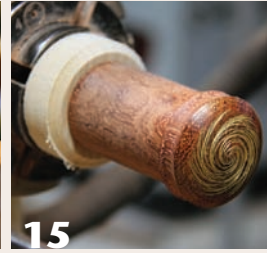
15 Jam chuck the outer box onto a waste block tenon to finish-turn the bottom.
