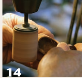
14 Carefully apply the inner tube to a drum sander to create the box's opening.
