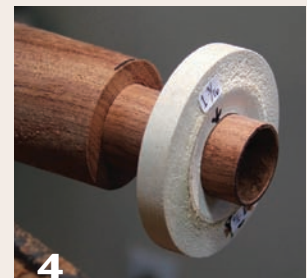
4 A simple gauge made by drilling the appropriate sized hole in scrap wood works well for checking your progress. Just slide the gauge over your workpiece (with the lathe off).
