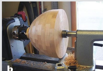
a A traditional ring-segmented bowl is turned, with an extra ring pressed (but not glued) to the rim with the tailstock. After it is turned flush, the extra ring is removed and cut into the shape of a basket handle.
