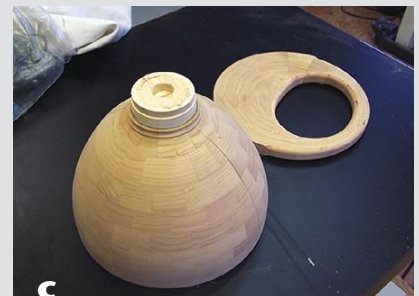
a A traditional ring-segmented bowl is turned, with an extra ring pressed (but not glued) to the rim with the tailstock. After it is turned flush, the extra ring is removed and cut into the shape of a basket handle.
