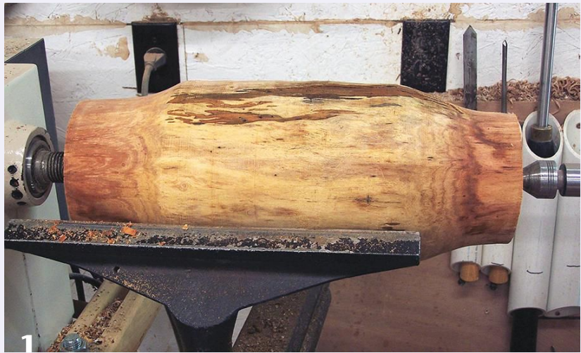
Starting with a mahogany log 18" long, the author turned the outside profile of an oblong bowl, knowing the piece would eventually be cut in half to make two identical bowls. He also turned a tenon at each end.
