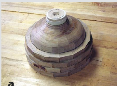
a A traditional ring-segmented bowl is turned, with an extra ring pressed (but not glued) to the rim with the tailstock. After it is turned flush, the extra ring is removed and cut into the shape of a basket handle.
