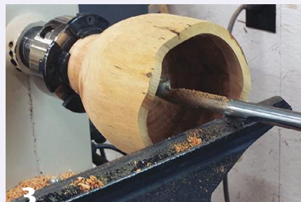
Each end is mounted on the lathe in a chuck and hollowed.
