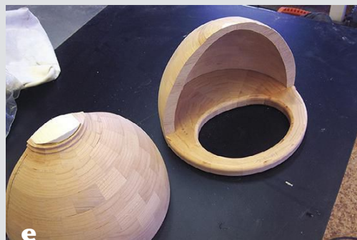
The segmented bowl is cut in half at the bandsaw, flat rim registered safely against the bandsaw table. Then the two halves are reassembled with the handle in the middle.
