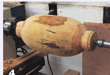
The two hollowed halves are glued back together, resulting in a fully enclosed oblong hollow form.
