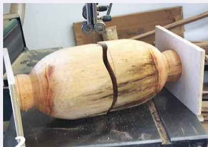
The turned form is cut in half crosswise at the bandsaw. Note the square plywood pieces attached to the ends for safe cutting.
