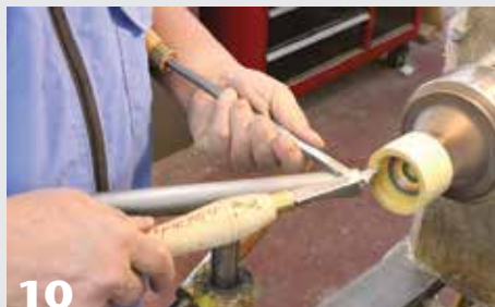
The female thread chaser is used with the armrest tool to form interior threads. An initial groove in the chamfer acts as a starting point for cutting the threads. Note that the chaser tool progresses to parallel with the bed ways as the threads develop.
