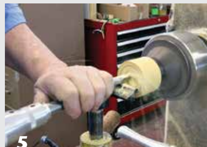
A solid prototype is useful for transferring diameters using a caliper. The pencil line on the endgrain shows a target diameter for hollowing the lid.
