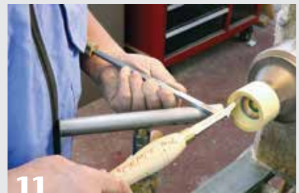
The female thread chaser is used with the armrest tool to form interior threads. An initial groove in the chamfer acts as a starting point for cutting the threads. Note that the chaser tool progresses to parallel with the bed ways as the threads develop.
