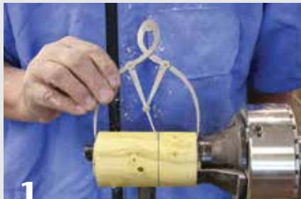
1 A golden mean caliper offers good proportions for a lidded box. Part the base from the lid, which remains in the chuck.
