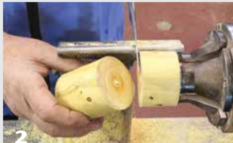
1 A golden mean caliper offers good proportions for a lidded box. Part the base from the lid, which remains in the chuck.
