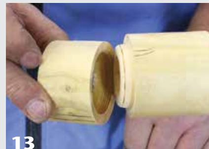
13 Use the lid to create a rub mark on the tenon, which offers a good indication of the crest of the male thread.
