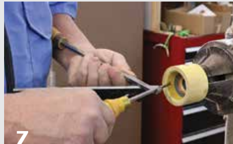
The armrest tool (in the author’s left hand) provides cutter access (right hand) inside the lid without having to position the toolrest perpendicular to the lid opening. Form a chamfer at the outer edge, then a recess where the threads will stop.
