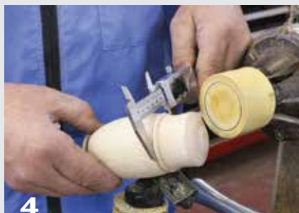
A solid prototype is useful for transferring diameters using a caliper. The pencil line on the endgrain shows a target diameter for hollowing the lid.
