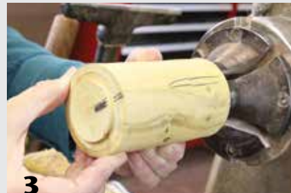
Hold the base up to the lid with the grain aligned and make registration lines to help with realignment later.
