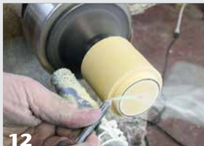
12 Form a tenon on the box base, and transfer the female thread crest span to the end of this tenon (pencil mark).
