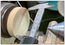
With the lid mounted in the chuck (bottom facing the tailstock), transfer the caliper measurement to the lid. This
