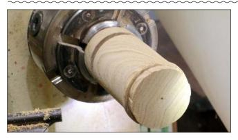
Test to see if the tenon fits into the hollow you just cut in the lid. If you stopped short of the caliper line, it should not fit yet.
