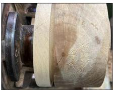
Check the fit by bringing the box up to the lid. If it doesn't fit over the tenon, use the parting tool to reduce the diameter a bit at a time until it
