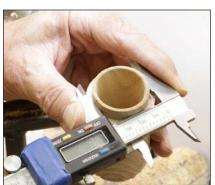
Measure the outside of the tenon with a Vernier caliper.
