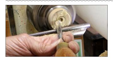
Remove the wood from the center of the lid working from the hole in the center to just shy of the caliper line. Here I use a 3/8" spindle gouge.
