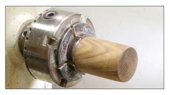
Re-chuck the box and use it as a jam chuck to hold the lid. Finish turning the top of the lid. To finish the bottom of the box, reverse its orientation on the lathe and gently clamp the tenon on the top of the box in the scroll chuck. If you are concerned about marring the tenon, wrap a layer of shop towel around it before snugging the chuck jaws. Bring up the tailstock and engage the live center. Take light cuts to remove the bottom tenon, and finish the bottom.
