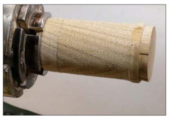
The box should fit snugly onto the lid and the edges meet squarely (note the joint faintly visible as a pencil line near the jaws). A bit of wax can be applied to the tenon and the inside of the lid but do not sand the tenon or the lid unless it is too tight to remove easily. If the lid will not pull straight off, twist it as you pull it apart.
