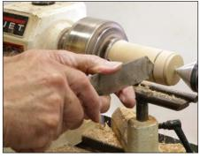
Determine the length of the lid, remembering that the tenon on the box will come up into the mortise on the lid. Because the lid will be grasped
