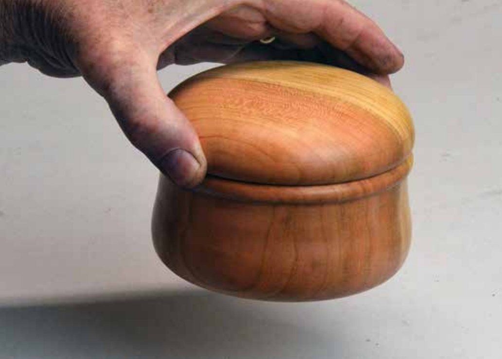
Hidden magnets hold the lid on this crossgrain box but pop it off when the lid is rotated to repelling polarity.
