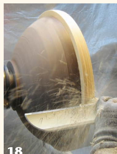
A parting tool is perfect for removing the center part of the rim material, which can be used on another, smaller bowl.
