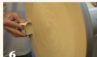
6 Prepare the gluing surface of the rim material with whatever method works best for you.
