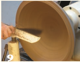
9 Remount the bowl into the 4-jaw chuck and turn the rim dead flat in preparation for gluing on the rim material.
