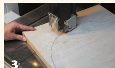
2 Measure, mark, and then cut the rim material to approximate diameter. Mount the rim material onto the lathe.
