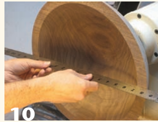
9 Remount the bowl into the 4-jaw chuck and turn the rim dead flat in preparation for gluing on the rim material.
