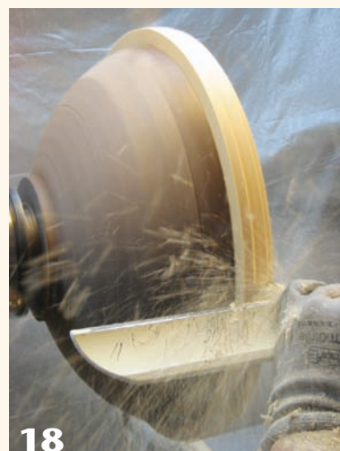
17 A parting tool is perfect for removing the center part of the rim material, which can be used on another, smaller bowl.
