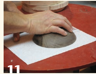
11 Minor adjustments to the bowl's rim and to the rim material can be made by hand sanding against a surface you know is flat.
