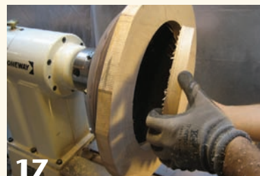
17 A parting tool is perfect for removing the center part of the rim material, which can be used on another, smaller bowl.
