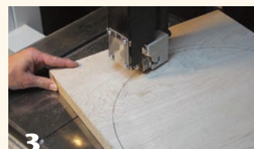
2 Measure, mark, and then cut the rim material to approximate diameter. Mount the rim material onto the lathe.
