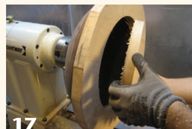
A parting tool is perfect for removing the center part of the rim material, which can be used on another, smaller bowl.
