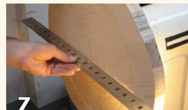
7 Use a straightedge across the entire diameter to test for flatness, not only at the rim area, but also across the entire board. It may be helpful to shine a light from under the straightedge to highlight any gaps.
