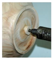
**Photo** 6 Turning the inside of the foot ring Carved Feet Made Simple - ©
