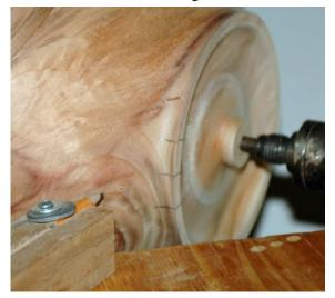
Photo 8 Mark the location of the feet on the ring
