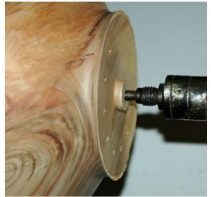
Photo 5 Use of centering pin for reverse turning
