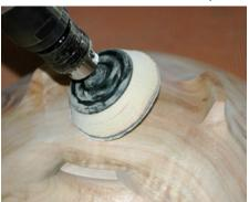
**Photo** 18 Sand with 120 grit on firm pad Carved Feet Made Simple - ©
