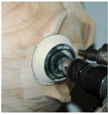
**Photo** 14 Start sanding with 120 grit on firm pad Carved Feet Made Simple - ©
