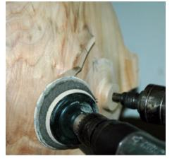
Photo 15 Finish sanding to 320 with soft pad
