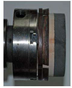
Photo 4 Use of rubber pad for reverse turning
