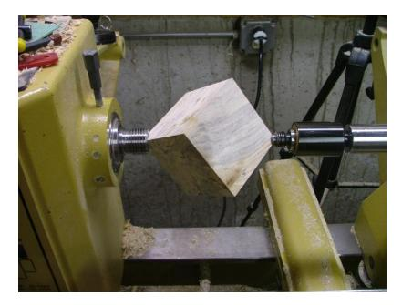
2. Before tightening the piece all the way verify the blank is being held squarely between centers. Place a piece of tape on the tool rest and use a pencil line aligned with one of the points (on the headstock side) and slowly rotate the piece using the hand wheel, check each corner and align as needed then tighten the piece down COMPLETELY and lock the tailstock in place.
