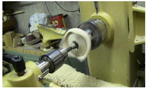
8. Hollowing is the next step. Using your favorite hollowing tool open the inside to about a 1/8" or even a little thicker. Due to its odd shape it is not a bad idea to leave the bottom a little thicker to allow it to sit and not wobble. Watch those wings while hollowing! Once hollowing is complete, use a pad sander to clean up the wings
