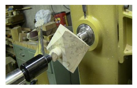
4. Once you have completed the initial shaping, turn the piece around and mount it in the spigot jaws using the previously marked centers to center the piece. Begin turning the top of the piece.
