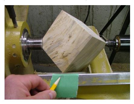
3. Now at the tail stock end using either a skew laying flat or a square scraper turn a tenon. Leave sufficient mass to be able to be held by the spigot jaws making certain to leave a square shoulder. The tenon should be about an inch around and 1-1/2" long. Now is also a good time to start shaping the bottom and removing the bulk of the material and the extra corners at the bottom.
