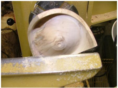
7. Drill a hole to a depth that suits the piece you are creating. For the pieces that I have created a depth of 1-1/2" is about right. Watch the tip of the bit and err on the side of caution, you can always hollow it out but you can't add.
