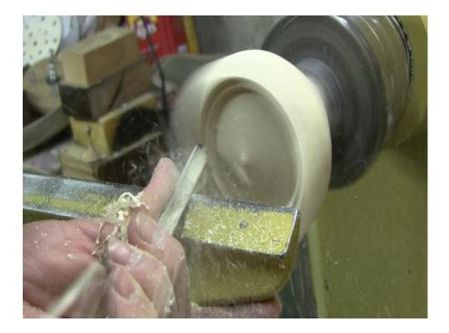
6. Turn the center down to match the shape of the bottom half of the box leaving an indent in the center to allow the Forstner bit to start.
