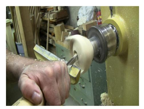
9. Now it's time to finish the bottom of the piece. Using a jamb chuck, reverse the piece and bring up the tailstock for support. Leave the tailstock in place for as long as possible to maintain support of the piece, finish shaping the outside. Sand and finish with you favorite sealer and finish.
