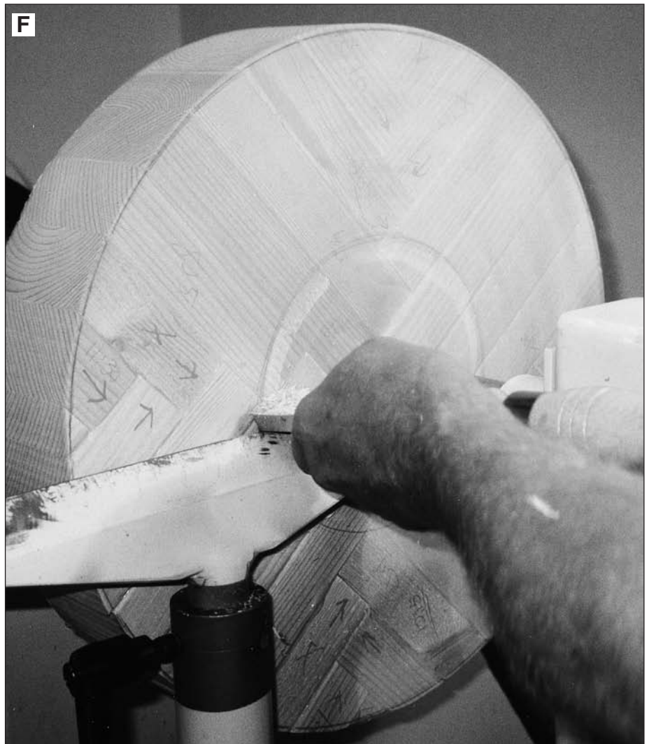
To ensure a solid mounting surface, turn a 6"-diameter flat spot in the assembly with a scraper as shown above. For this step, wedge the blank against a 14" flat plate attached to the head stock using a live center in the tail stock.
