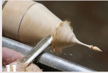
11 Restore the taper to meet the section for the elongated vase.
