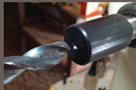
21 Drill the arbor blank to receive a bearing insert.
