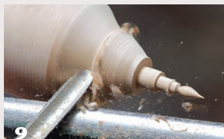
9 Restore the taper on the stock to meet the new \frac{3}{8} " working section.
