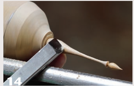
14 A planing cut with the skew chisel further defines the vase shape.
