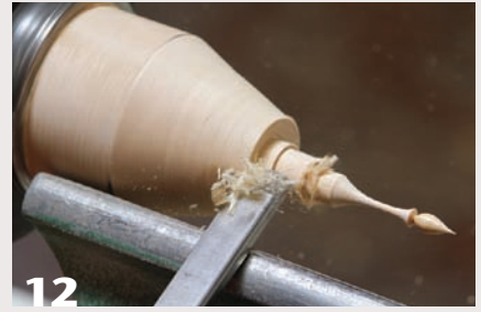
12 A peeling cut with the skew chisel begins to define the vase shape.
