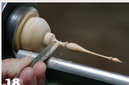
18 Use a \frac{3}{8} " spindle gouge to cut the cove.
