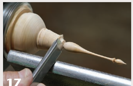
17 Make a V cut with the long point of the skew chisel to define the vase-to-cove transition.
