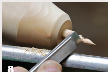
8 Using the long point of the skew chisel, define the intersection of the flame tip and saucer.
