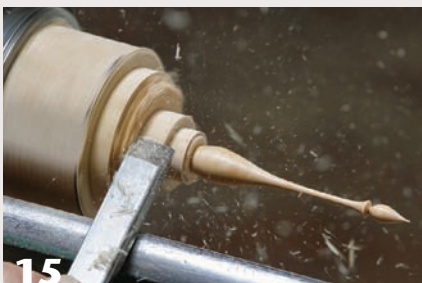
15 A peeling cut with the skew reduces the stock diameter for the next cove.
