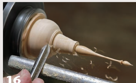
16 Form the base of the finial using a \frac{3}{8} " spindle gouge.
