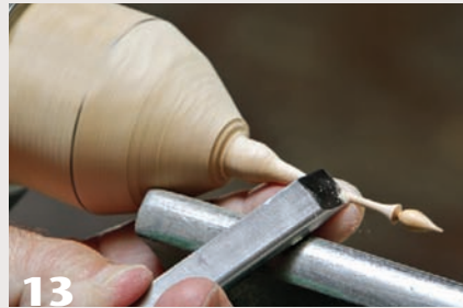
13 A planing cut with the skew chisel showing finger support for the thin shaft.
