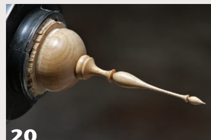
20 The completed finial before parting off the lathe.
