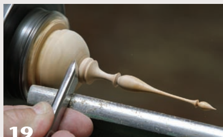
19 Define the intersection between beads with the skew chisel.
